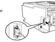
**3** Connect the other end of the cable to the parallel port on the back of your computer.
